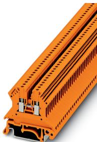
Feed-through terminal block, nom. voltage: 500 V, nominal current: 17.5 A, connection method: Screw connection, number of connections: 2, cross section: 0.14 mm<sup>2</sup> - 1.5 mm<sup>2</sup>, AWG: 26 - 16, width: 4.2 mm, color: orange, mounting type: NS 35/7,5, NS 35/15, NS 32
