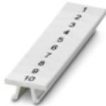
Zack marker strip, Strip, white, labeled, Printed vertically: consecutive numbers 1 ... 10, 11 ... 20, etc. up to 91 ... 100, mounting type: snap into tall marker groove, for terminal block width: 4.2 mm, lettering field size: 4.2 x 10.5 mm, Number of individual labels: 10
