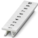
Zack marker strip, Strip, white, labeled, printed horizontally: consecutive numbers 1 ... 10, 11 ... 20, etc. up to 91 ... 100, for terminal block width: 4.2 mm, lettering field size: 4.2 x 10.5 mm, Number of individual labels: 10
